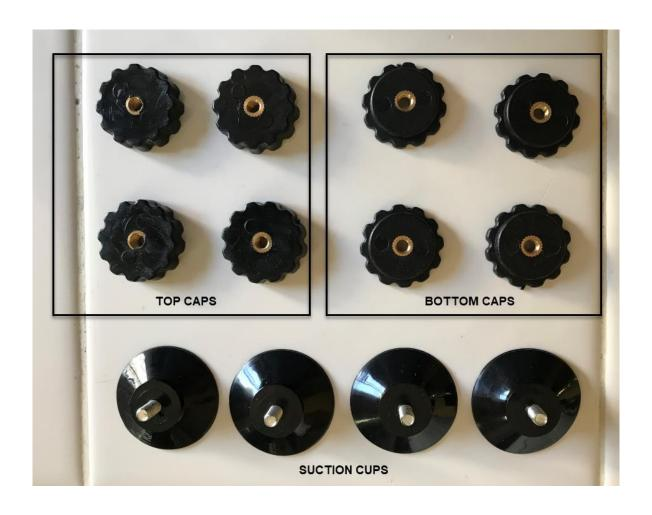
**Step 2** Screw bottom cap to suction cup until it bottoms out as shown below. Do not over tighten. Repeat 3 more times to make 4 complete sets.
